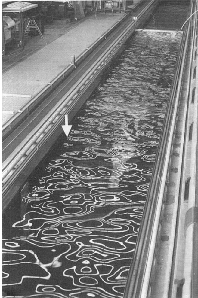
FIGURE 6. Surface appearance of flow in primary cell (rough) and outside (smooth) for the case of a plume-driven flow. (Cell boundary indicated by arrow.)
